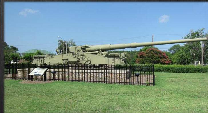
The T1 240 mm prototype gun on T72 carriage, cannibalizing parts of Anzio Annie , the M1 Howitzer, and the M1 Gun.
