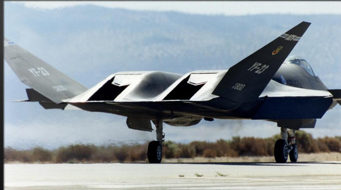
Rear view of the YF-23 displaying embedded engines and shielding.
