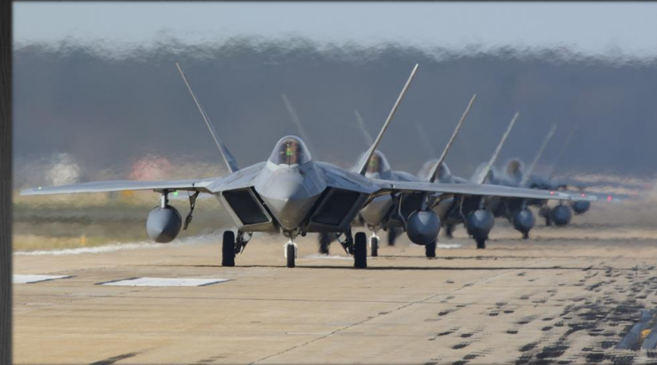
F-22's during an elephant walk, note the external fuel tanks exhibiting the F-22's add-on external pylons.
